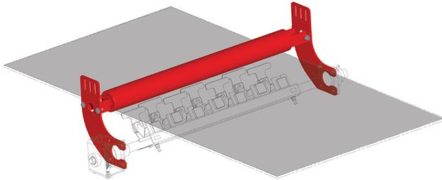
Martin® Pressure Roller Brackets provide firm support for the belt line over a secondary cleaner allowing effective cleaning. Available with new return rollers or use existing equipment. Mounts to conveyor stringer with three bolts or may be welded in place.
